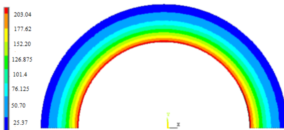
Fig.7. Static loading – Nodal solution showing von Mises stress distribution at internal pressure of a) 4.83MPa
